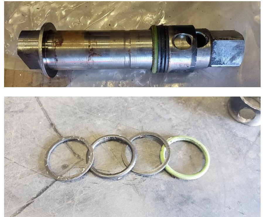
The valve internals after test
